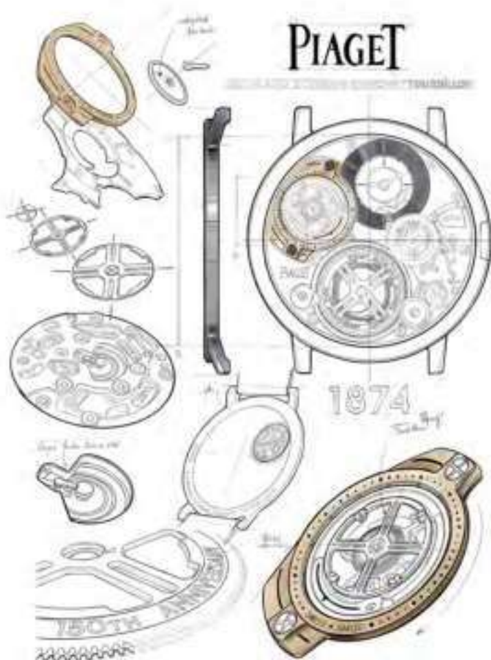
About 90% of the components of the Altiplano Ultimate Concept had to be redesigned to accommodate a flying tourbillon in the new model
